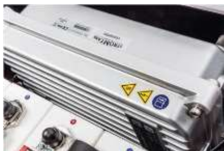
The power supply electronics are constructed in a shielded cast housing
